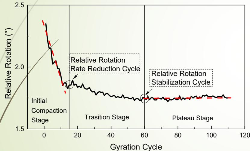
**Stage I : Initial compaction stage**
