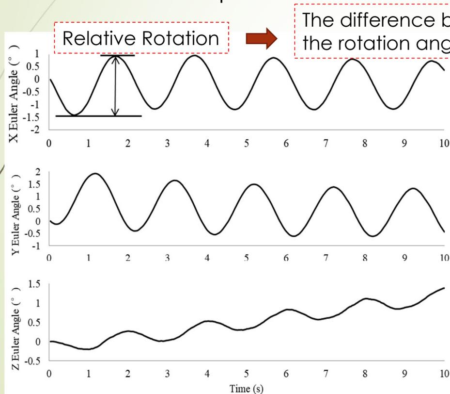
Particle follows a **cyclic rotation pattern** that repeats every 2 seconds that matches the SGC rotation speed of 30 rpm.
